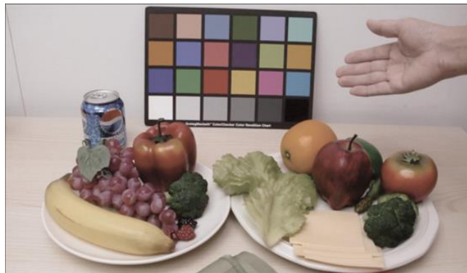
Figure 5. Colour Rendering Index (CRI) comparison. Image courtesy Gerben49 via Wikimedia Commons.
