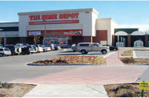
Figure 4.9.1. When complete separation of pedestrians from movement of vehicles is not possible, site plans should minimize hazards by using special paving, landscaping, and other means to clearly delineate pedestrian areas.
