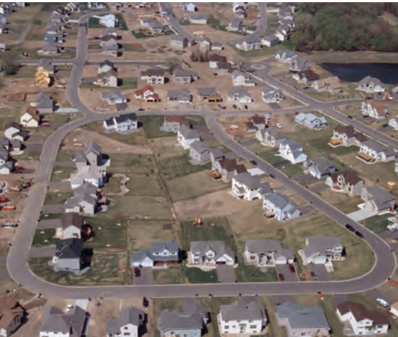
Figure 4.11.1. A limited-access street design provides this residential subdivision with few points of entry or exit.
