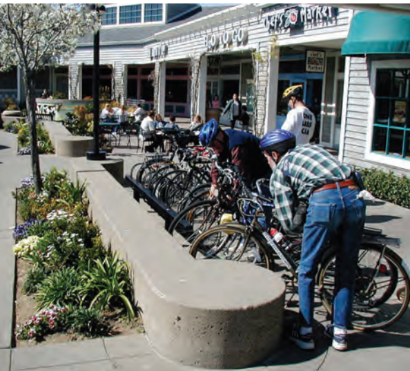
Figure 4.9.2. Bicycle parking should be located close to building entrances yet where it will not impede pedestrian or automobile flow.
