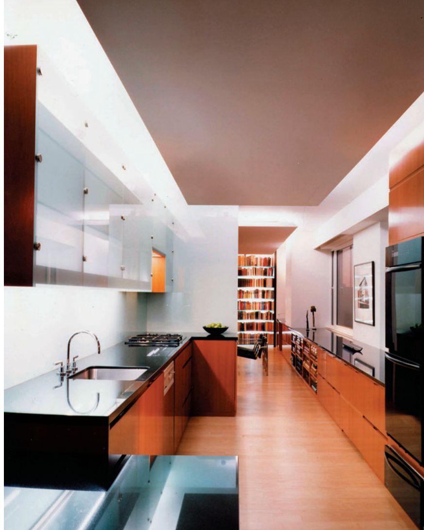
The kitchen of this apartment is primarily lit with fluorescent tubes. The upper cabinets are backlit with fluorescent lighting. Ling expanded the same dropped ceiling treatment into the kitchen where he could conceal indirect fluorescent lighting in the soffits. Since the apartment is layered with fluorescent lighting, it creates a balanced and comfortable effect for the eye, even when viewing the library from the doorway of the kitchen.
